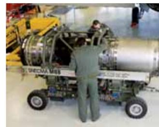
incorporates advanced technologies such as integrally-bladed compressor disks, called 'blisks', low-pollution combustor, single-crystal high-pressure turbine blades, ceramic coatings, revolutionary powder metallurgy disks, and composite materials. Additionally, the M88 has been optimised so that its small infrared signature does not compromise the Rafale's overall IR signature, and its non-polluting, smoke-free emissions make the aircraft more difficult to detect visually than older designs.
