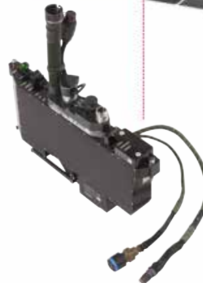
Oxygen regulator and anti-G system
